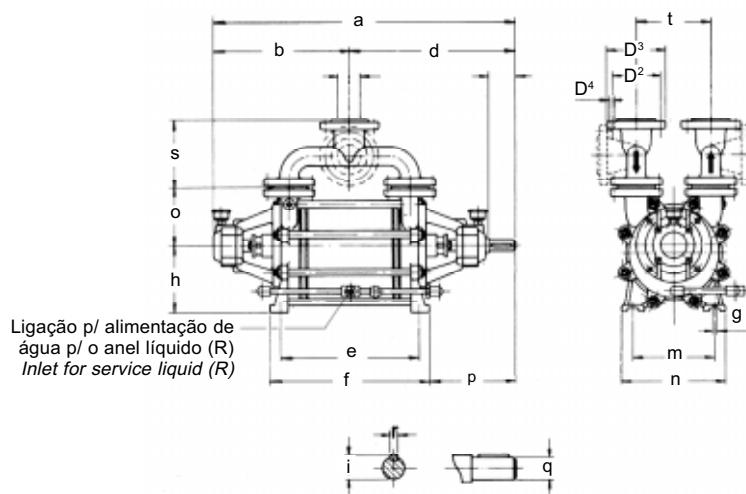
Bomba tipo BLN/MV 380 a 910/Pump types BLN/MV 380 to 910
